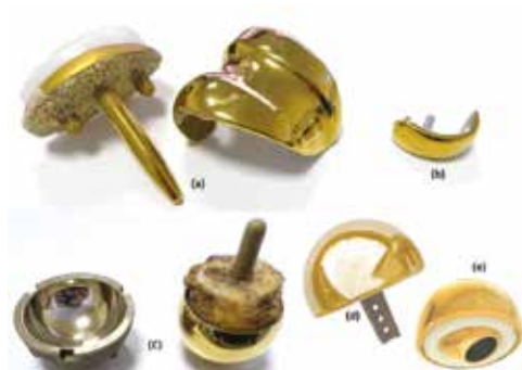
Figure 2: Three retrieved femoral heads coated with titanium niobium nitride. Coating removal is macroscopically visible on all heads [5].
